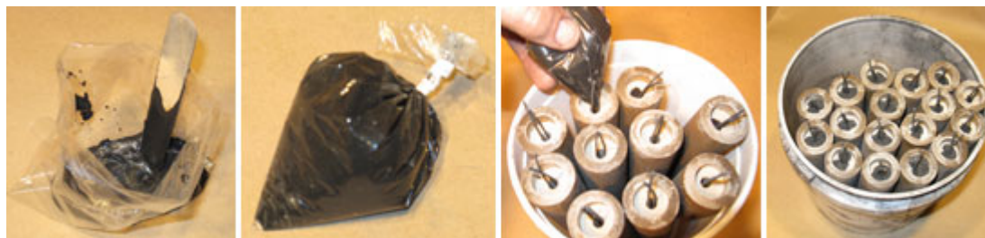
Priming the Gerbs with Black Powder Slurry
