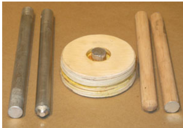
Finished Homemade Gerb Tooling, With Aluminum and Wood Rammers
