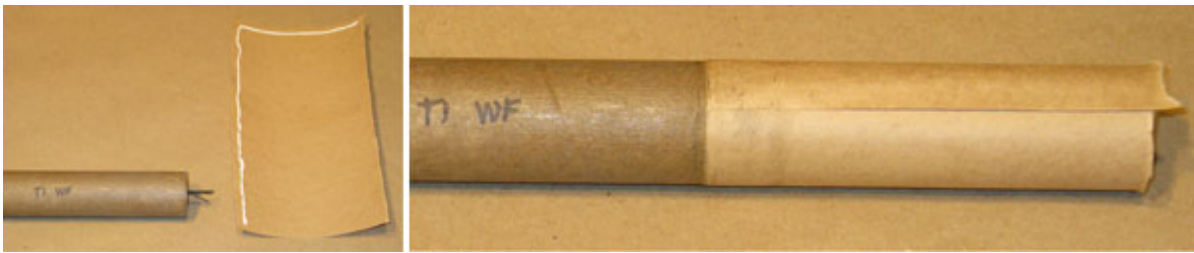
Installing Paper Buckets on Gerbs
