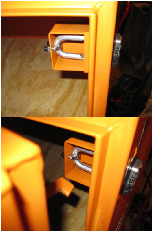
Installation of Lock in Ridgid Jobsite Storage Box
