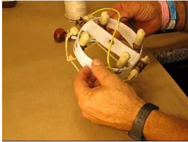
Fast-Visco Fuse and Green Ignition-Visco Fuse Installed on Girandola
