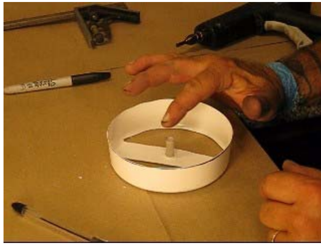
Hot-Gluing Tube into Hole in Girandola Frame
