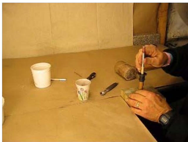
Ramming Fuel in a Magnum Bottle Rocket Motor
