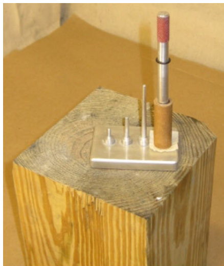
Tooling Ready to Ram Clay Plug
