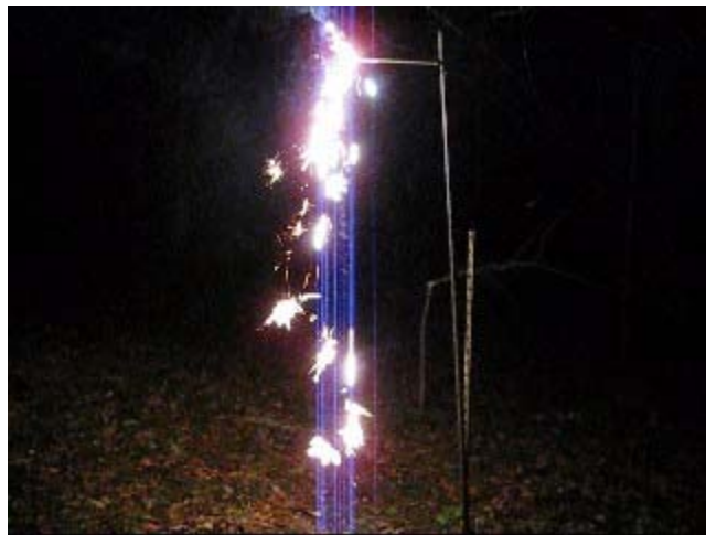
A Tube Sparkler Made with Coarse Spherical Titanium Metal
