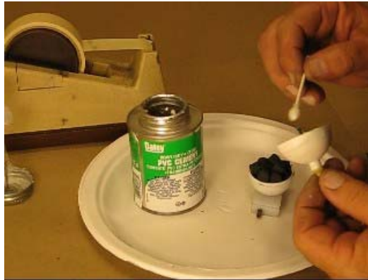
Applying PVC Cement to Shell Casing with Q-Tip
