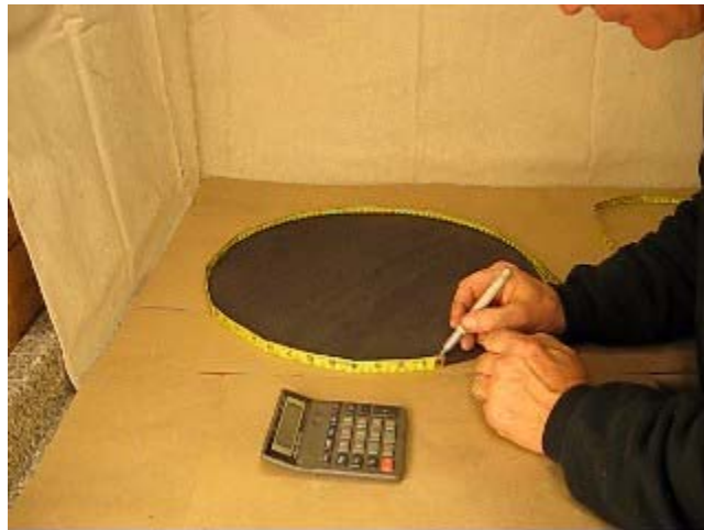
Measuring and Marking Frame for Driver Locations
