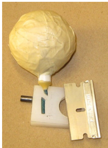
Cutting Visco Time Fuse at a Sharp Angle
