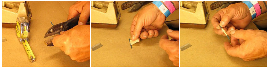
Cutting and Tape-Wrapping Visco Time Fuse
