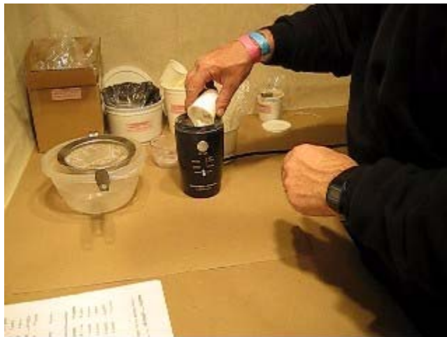
Pulverizing Chemical in a Blade-Type Coffee Mill
