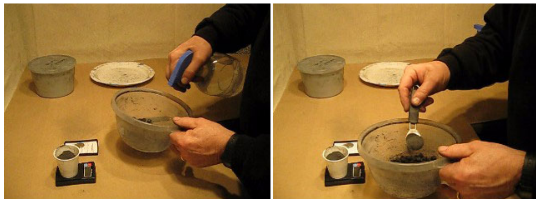
Spraying Stars with Water, and Dusting with Black Powder Prime
