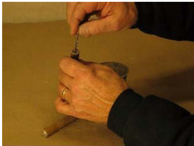
Hand Twist-Drilling 1/8-Inch Bulkhead Passfire Hole
