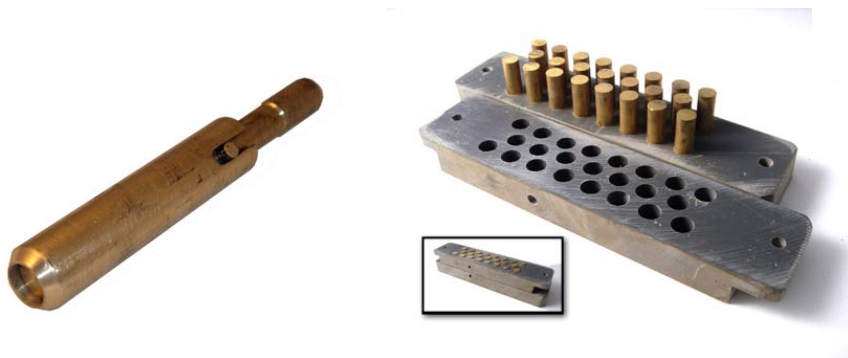
3/8-Inch Brass Star Pump and Star Plate
