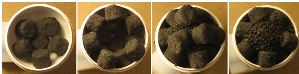
Filling Shell Half with Stars and Break Charge
