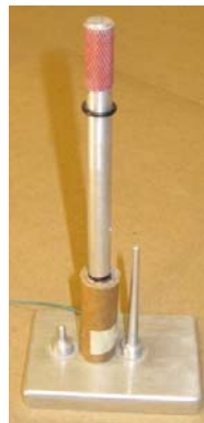
Marking Solid Rammer at Top of Tube
