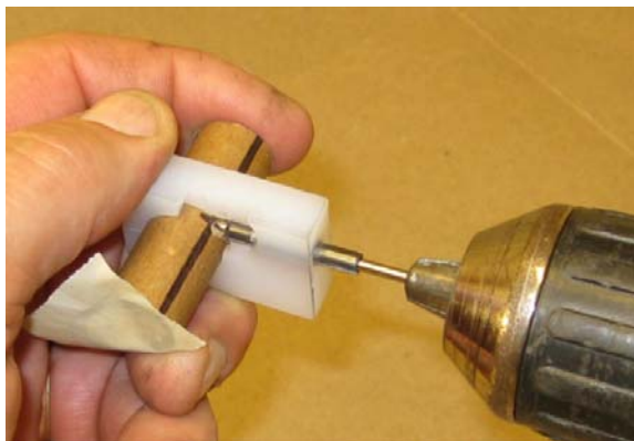
Drilling Hummer Spin Hole with 3/32-Inch Bit and Drill Guide
