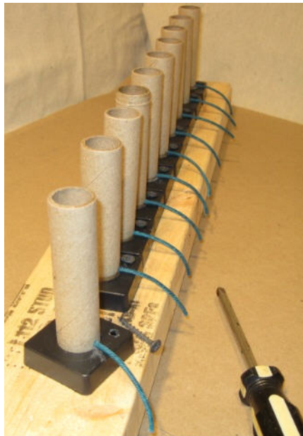
Attaching Mortars to 2x4 Board
