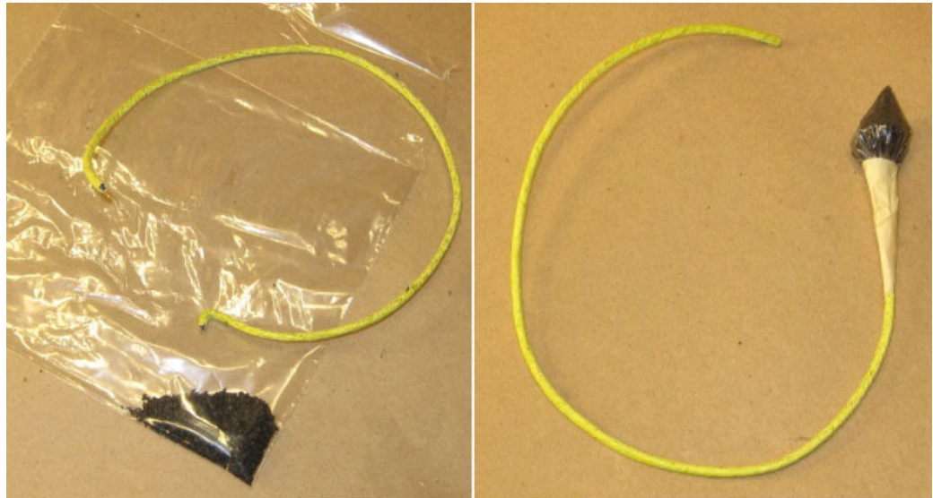
Assembling Lift Powder Baggie and Shell Fuse Leader
