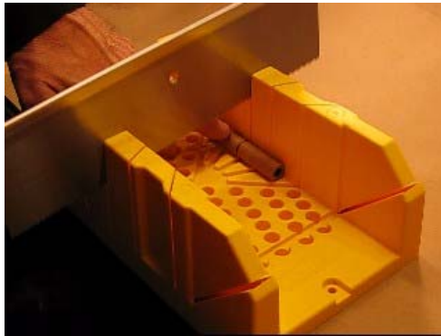
Cutting a Paper Tube in Half with Hand Miter Box and Saw
