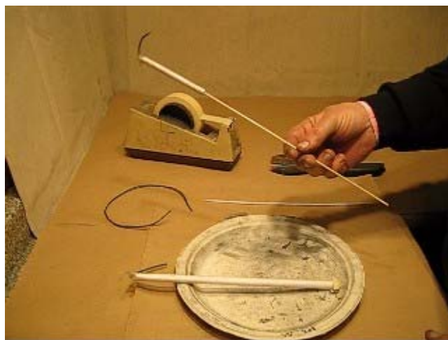
Attaching Fuse and a Handle to the Sparkler
