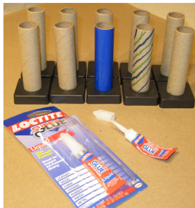
Gluing Mortar Tubes into Plastic Bases
