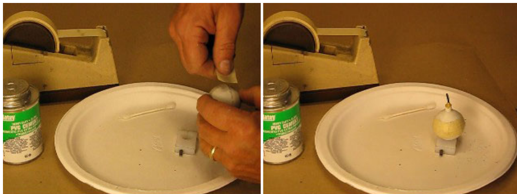
Applying Masking Tape over Glued Shell Casing Equator
