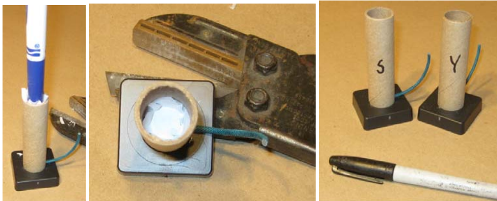
Pushing 1.5-Inch Paper Square Down on Top of Fish Fuse, Marking Mines for Future Identification
