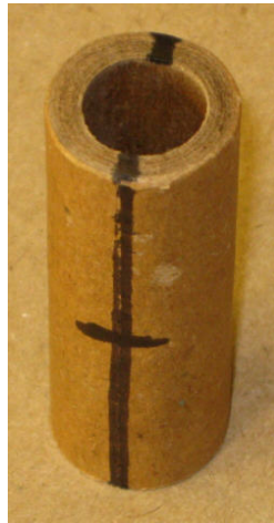
Marked Hummer Spin-Hole Location (Same Mark on Both Sides of Tube)
