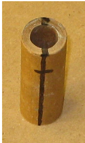
Marked Whirlwind Hole Location (Mark on Line on Other Side is 3/8-Inch from Other End)
