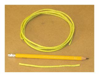
Super-Fast Paper Fuse. Three thin strands of blackmatch, wrapped in tissue paper, 1/8-inch diameter paper fuse (1/16-inch diameter blackmatch strands). Paper-wrapped fuse burns at about 1 second per foot. Skylighter #GN1205. Quantity needed—10 feet of paper-wrapped fuse (yields 30 feet of thin blackmatch)
