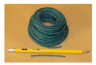
Thin Chinese Visco ignition fuse, 1mm (3/64-inch) diameter. Green fuse, burns at about 5 seconds per inch. <a href="Skylighter#GN1010">Skylighter#GN1010</a>. Quantity needed—3 feet
